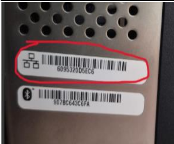
Photo 1: MAC Address is typically on a sticker on the back next to the network box symbol. Can also be obtained by checking Network settings. Use the Wired MAC Address.
